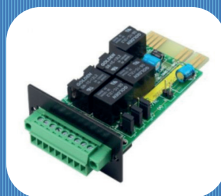
DRY CONTACT Contactos seco
