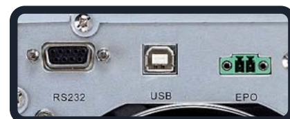
External communications/emergency shutdown ports
