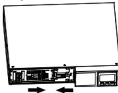
Re-connect the battery wires.
