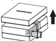
Remove the top cover of battery box and replace the inside batteries.
