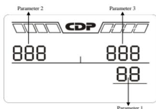
There are three parameters to set up the UPS. Parameter 1: It's for program alternatives. Refer to below table. Parameter 2 and parameter 3 are the setting options or values for each program.
