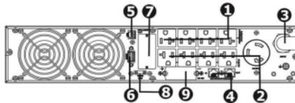
1. Programmable outlets: connect to non-critical loads.
