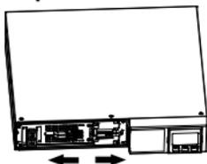
Disconnect battery wires.
